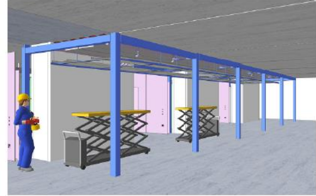
Once secure, support can be removed and the process repeated
